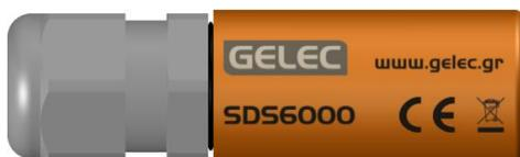
The Seam Detector Sensor SDS6000 is a part of the Seam Detection System, which is commonly used in fabric dyeing machines. Having an innovative and latest technology magnetic sensor, it maximizes the detection efficiency. It is compatible with the Seam Detector Unit SDU6000. It should be mounted externally on the machine close to the fabric path (up to 30cm), which has a magnet (MSD05 - Ø8x40mm) sewed on its seam.
